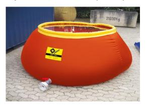
The open water tank is self- erecting thanks to the float ring. The tanks, which are made of tear- proof PVC, have a very sturdy anodised 2" aluminium flange and a shockresistant PVC ball valve. The tank can be filled and emptied with speed and ease using a Storz C coupling. Vetter supplies the water tanks with repair kit as standard and until 5,000 l in a practical packing bag.
