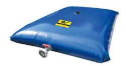
Reinforced PVC gives the closed water tanks maximum stability. You can also opt to have corner brackets fitted to the tanks for safe transportation by truck - even of filled tanks. An opening on the top side of the tank serves as a vent or for refilling.
