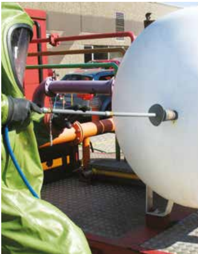
Seal leaks from a safe distance
