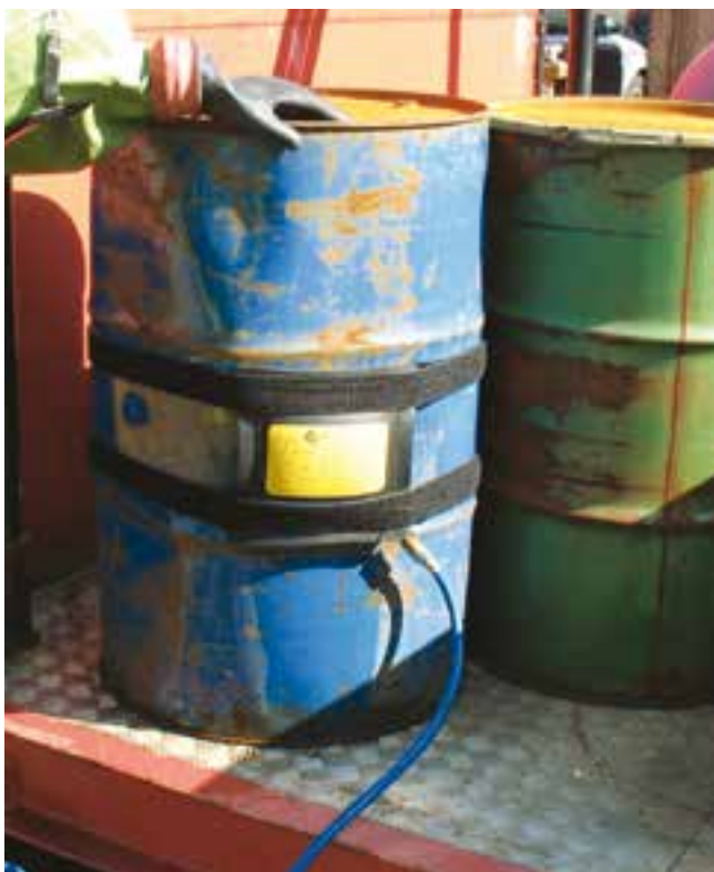
Sealing bags stop leaks in drums
