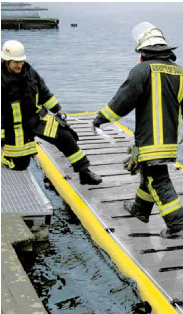
Safe walkway due to the anti-slip strips
