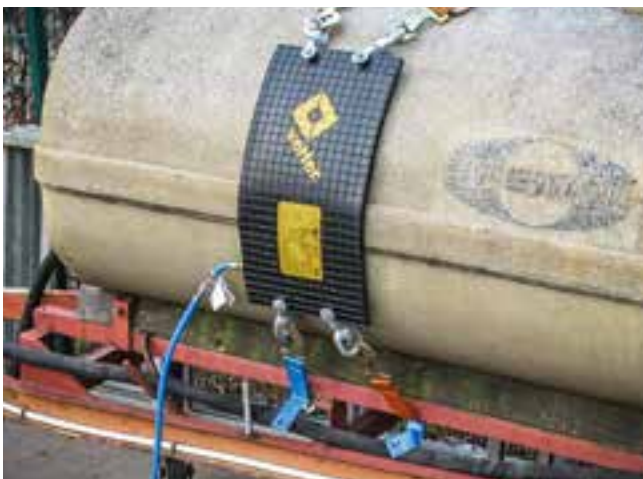
Leak sealing bags with swivel eyes
