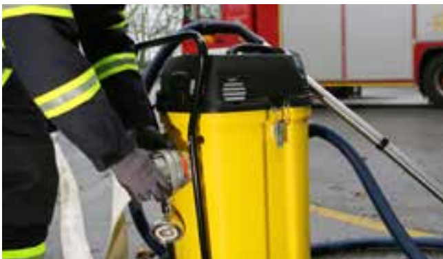
Connection for fire-service hose
